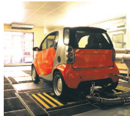
48" Emission Chassis Dyno – single axis design with automatic vehicle fixation
