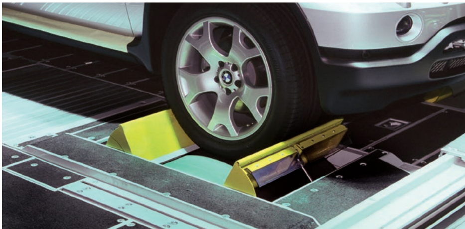
48" Emission Chassis Dyno – single axis design with automatic vehicle fixation
